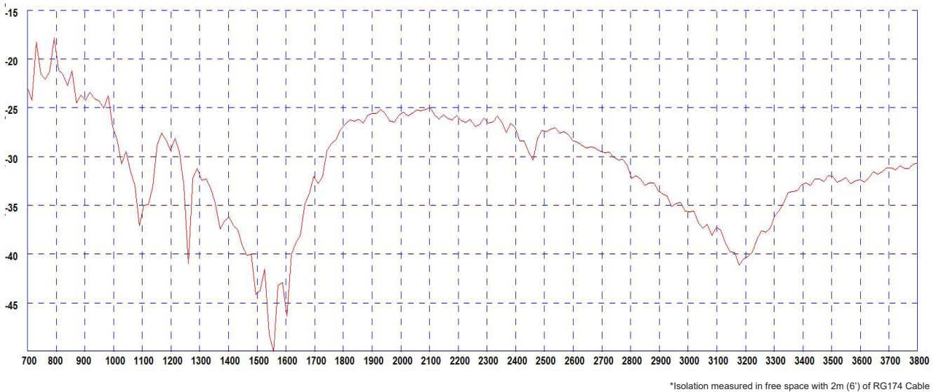
Typical Isolation Elements 1&2*
