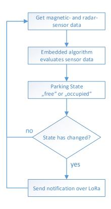
The sensors data are processed by the devices embedded algorithm. The algorithm output is the parking state "free" or "occupied". The device checks, if the parking status has been changed since the last processing run and in case the parking state change will be communicated via the LoRa interface. This means, that the parking sensor will only report, if the parking state has changed.
