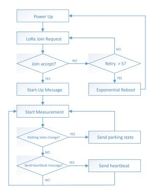
The parking state message can be configured as not confirmed with or without repetitions. This reduces the use of duty cycle to acknowledge all messages, but may also reduce the percentage of successfully received messages by the Gateway.
