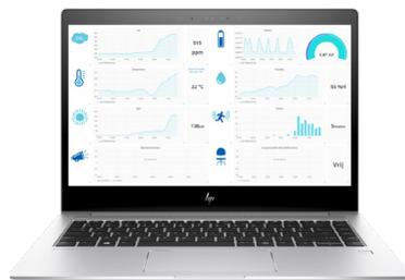
In the application you can directly view the CO<sub>2</sub> values in clear dashboards. In addition, you will also receive alarms if the CO<sub>2</sub> values exceed a threshold (self-adjusted limit values).
