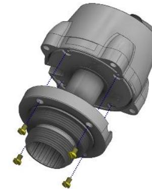
**Note:** This adaptor can also be used with the waveguide option but will require a 36mm pipe. The waveguide pipe should be securely attached via the two grub screws provided and hand tightened with an M1.5 Allen key (Note: over-tightening the grub screws can damage the plastic).
