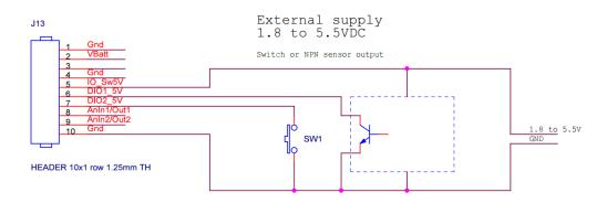
Pin6 is connected to DI1 this pin is also used for the RX of the terminal. Enabling DI1 will disable receiving anything from the terminal/debug tool. On the original cable this is the RED-wire
