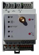
On a single-phase installation, the **TRIPHAS'O** sensor provides the energy and power absorbed on each circuit (submetering).
