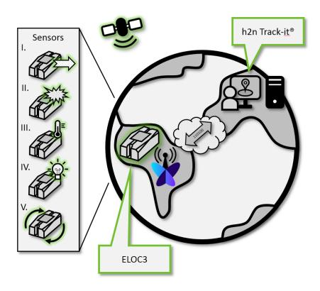
In order to ensure a most accurate tracking, the device waits until at least 5 satellites have been reached. If this state is not reached after a maximum of 40 seconds, the waiting process is aborted and the previously determined position, even if they are inaccurate, is used. If no positioning can be carried out, an error telegram is sent, which can be displayed in the h2n Track-it<sup>®</sup> cloud.
