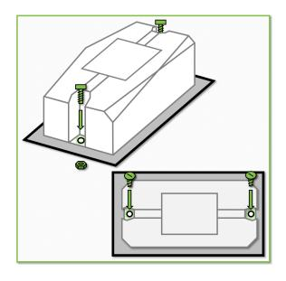
that no unevenness has occurred. Use two M4 screws, see **A)**, for the fixation. Insert the screws through the holes provided and fix them with a nut, see **D)**.
