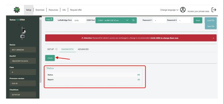
Press **Check** to verify the correct communication betweet the LoRaWAN® interface and the slave(s).
