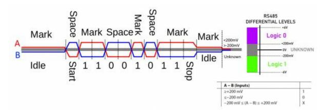
The objective of biasing is to make sure that the RS485 line remains in a known, non-fluctuating state when no devices are transmitting. Polarization of the pair must be implemented at one location for the whole serial bus. Biasing the entire network requires a single pair of polarization resistors: a pull-up resistor to +5V attached to the "+" signal line, and a pull-down resistor to ground attached to the "-" signal line.
