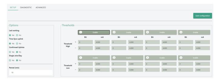
On the MCF-LW06424 is possible to set 4 thresholds for each channel:
