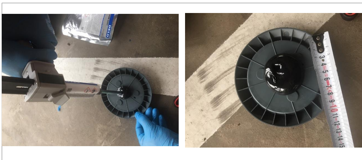
Figure 10 Application de la colle
