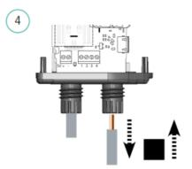
Once the cable has been removed, insert the gland plug provided in the package to maintain the watertightness of the product
