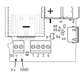
N.B.: To power the product via an external power supply it is nec-essary to disconnect a probe in order to pass the cable of the power supply in the cable gland.
