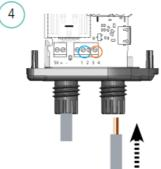
Insert the cable of the probe supplied with the product and connect the wires to the terminal blocks:
