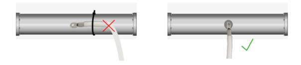
**WARNING**: the probe must be manipulated at room temperature, risk of damage if handled in negative temperatures or above 90°C
