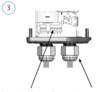
Using a suitable screwdriver, unscrew the terminal block to gland to loosen detach the wires the cable
