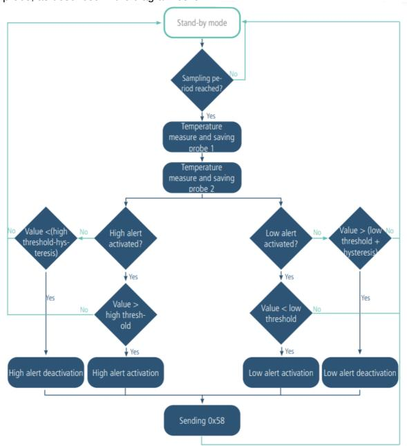
The sampling period (reading) enables to determine when the product will do the temperature measure and so the frequency at which the product will detect an overpassed threshold.
