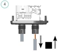
Once the cable has been removed, insert the gland plug provided in the package to maintain the watertightness of the product
