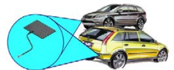
Typical antenna positioning
