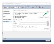
**Step 7:** Make sure the all the boxes Flash and EEPROM and Fuses are selected and that erase memory before programming and verify programmed content are ticked
