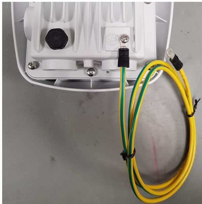
Figure 12: Earthing with mounting kit provided
