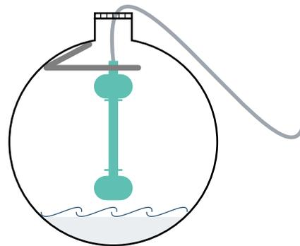
The double-level sensor is made of 304 stainless steel to be compatible with all types of non corrosive fluids. It can withstand a maximum temperature of 120 ° C and a maximum pressure of 5MPa (=50 bars).
