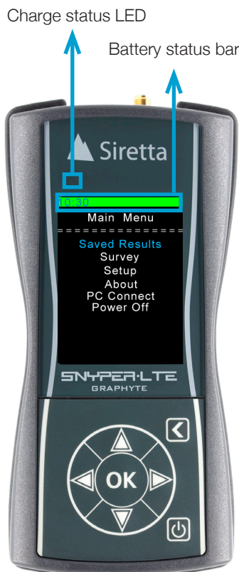
Figure 7. Charging and battery status
