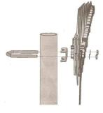
The single U bolt mounting allows the antenna to be adjusted in the vertical plane by approximately 26 degrees up and down from the. horizontal position.
