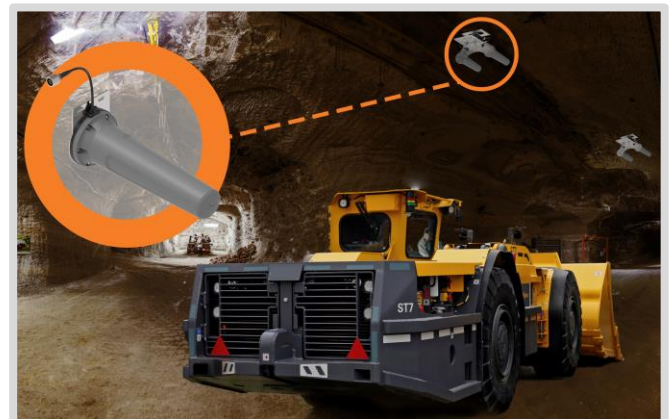
2x HELI-11 antennas mounted on the BRKT-45 for MIMO application
