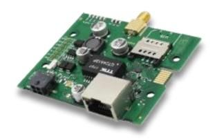
Small and quick to deploy industrial Ethernet to 4G LTE IoT gateway. Advanced VPN functionality, security and remote management capabilities makes TRB140 the best option for single device connectivity.
