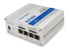
Next generation LTE-A Cat6 cellular IoT router with Dual SIM, Carrier Aggregation and Gigabit Ethernet interfaces. Rugged and powerful choice with VPN, Firewall and plenty of processing power for custom applications on OpenWrt based RutOS system.
