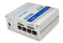
Next generation LTE-A Cat6 cellular IoT router with Dual SIM, Carrier Aggregation and Gigabit Ethernet interfaces. Rugged and powerful choice with VPN, Firewall and plenty of processing power for custom applications on OpenWrt based RutOS system.
