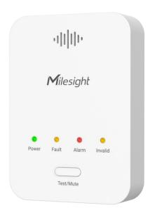
GS101 is a LoRaWAN<sup>®</sup> residential gas detector to detect the natural gas leak and send alarms. When the concentration caused by gas leak reaches the preset threshold, the detector will trigger both LED light alarm and buzzer sound alarm, it also supports controlling outputs to close the gas valve and open the vent fans to prevent potential accidents.
