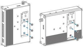
2. Hang the device to the DIN rail. The width of DIN rail is 3.5cm.
