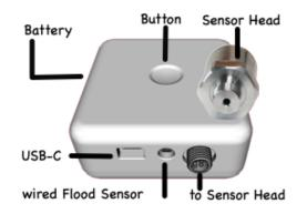
As soon as the unit is connected to a radio network, an automatic calibration begins. Use water normally during this time. After 24 hours at the latest, this calibration is finished. It is detected whether a pressure reducer is present, and which standard pressures are present in the water system. You can restart the calibration from the app if necessary (configuration menu).
