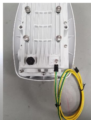
Mandatory ground connection on the Wirnet™ iStation
